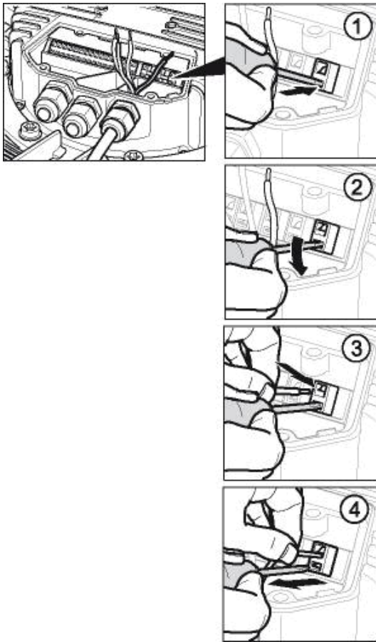
Fig. 2: Connecting the wires to terminals
