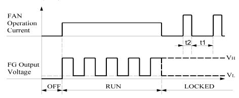
$\bigstar$  Electrical Characteristics : Vcc = 12V, (at Ta = 25°C)
