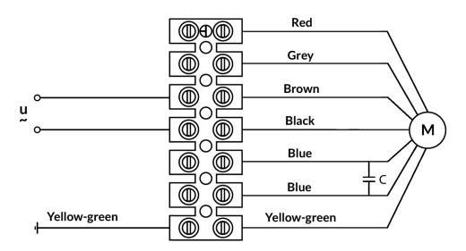
\* if you connect the live wire to the terminal red or grey, the fan will operate with lower rotational speed
